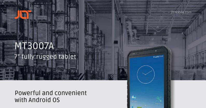
The MT3007A™ is a fully rugged tablet with Android™ operating system that is also very portable, making it ideal for long days of field service in warehousing operations and other harsh environments. It is IP65 dust-proof and waterproof and works in temperatures of -20°C to 60°C / -4°F to 140°F (AC mode), -10°C to 50°C / 14°F to 122°F (Battery mode)
