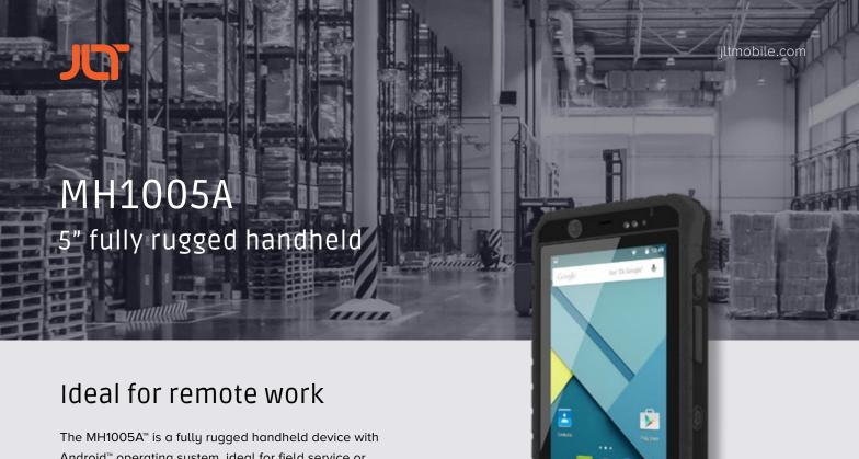
Android™ operating system, ideal for field service or warehousing operations in harsh environment. It is IP65 dustproof and waterproof and works in temperatures of -10 to +50 °C / 14 to +122 °F.
